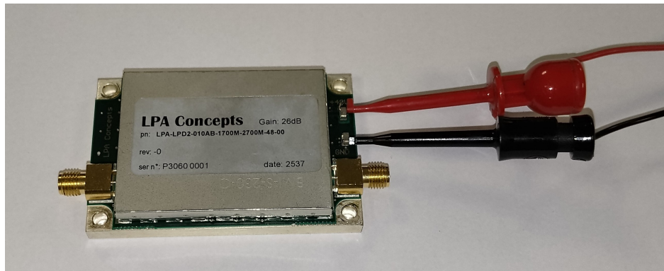
Figure 1 : Supply connection on LPD2 amplifiers
