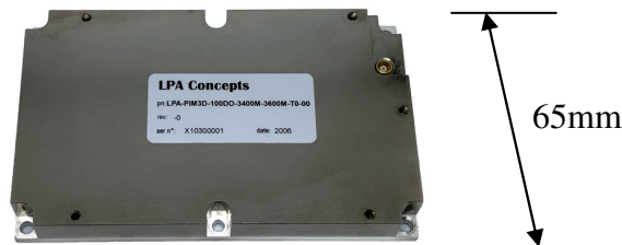
Band 42 TDD front end module with 250Wpeak Tx power
